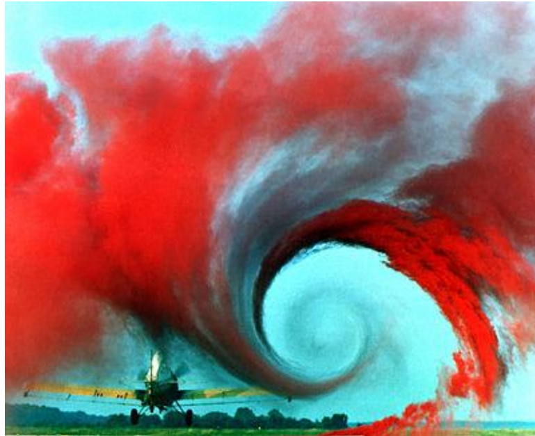
Figure 9 : Vortex created by the passage of an aircraft wing (Wikipedia, 2008)
